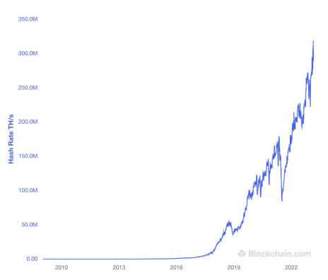
Figure 9. The collective hash rate in the Bitcoin network, in terms of the number of hashes that get computed per second (measured in terahashes, where 1 terahash =  $1 \times 10^{12}$  hashes). This graph was taken from <u>https://www.blockchain.com/explorer/charts/hash-rate - (Exhibit SM-18)</u>.
