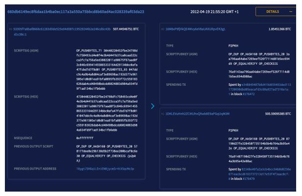
Figure 3. More detailed information of the same Bitcoin transaction as above. Notably, we can see the Bitcoin Script used, the address used in the input, and the transactions in which the outputs later spent their contents.
